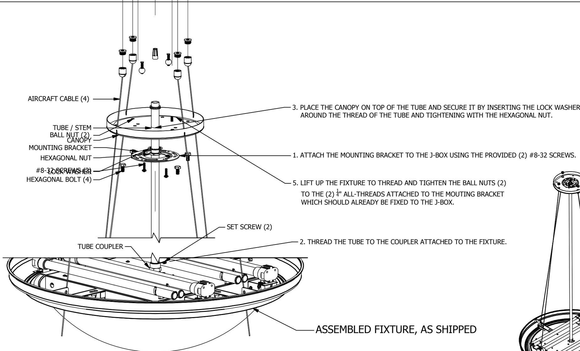
FIGURE A. FIXTURE COMPONENTS
